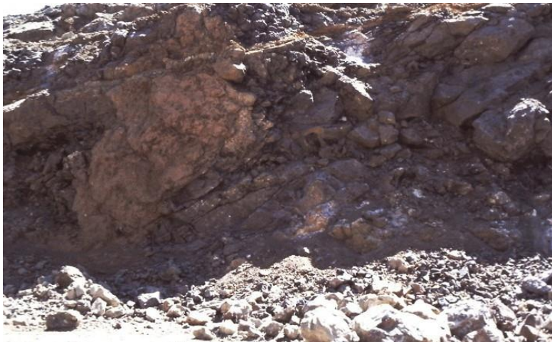
Figure 34. Large replacement remnant of carbonatite (light gray, left half of photograph) that has remained within fluorite ore (dark gray, right side of photograph), and it attests to the replacement process and that the replaced rock is carbonatite. B band, B open pit, Okorusu.
