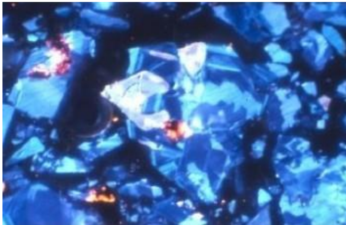
Figure 28. Apatite crystals (white, center of micrograph) partly replaced by fluorite (light to dark blue) in carbonatite-replacement fluorspar ore. During milling this intergrowth produces binary locked apatite-fluorite particles that carry deleterious phosphorus into the fluorspar concentrates. Note zoning (dark and light gray bands) of central fluorite crystal. Cathodoluminescence microscopic micrograph. 60X.
