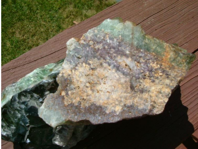
Figure 8. Hand specimen of green fluorite (medium gray, coarsely crystalline) deposited on top of purple fluorite (medium gray, fine grained). Purple fluorite had earlier been deposited upon potash feldspar (light gray). A band, B open pit, Okorusu Mine.
