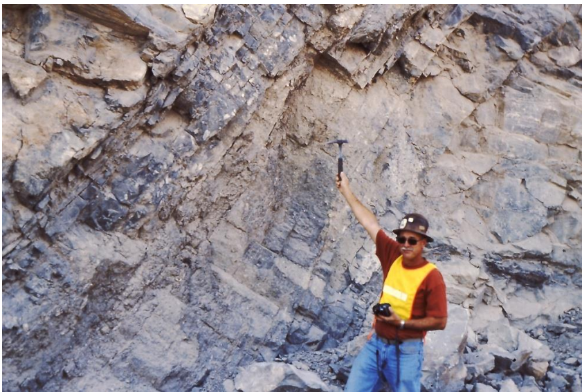
Figure 27. Tinguaitite dike (dark gray) traversing fenite (medium to light gray) in a mine heading at the B open pit, Okorusu mine.
