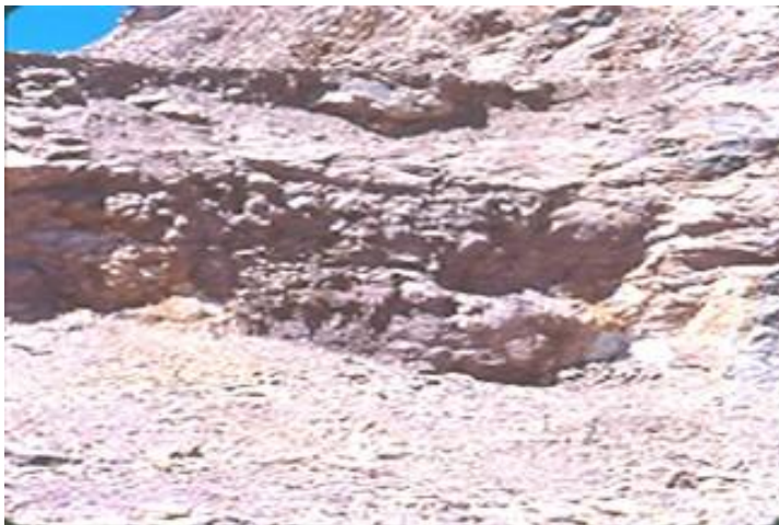
Figure 29. Fluorspar ore (center of mine face, horizontal banding) replacing marble to the right of the fluorspar orebody. A band, B open pit, Okorusu mine.
