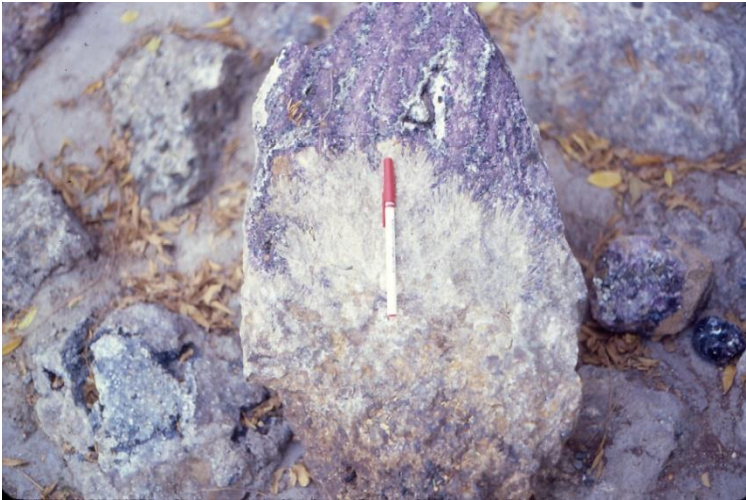
Figure 16. Hand specimen showing abundant apatite (white, beneath pen) as radial acicular crystals in fluorite (medium gray) ore. Apatite crystallized as a component of carbonatite and remained in the fluorspar as an insoluble constituent upon replacement by fluorspar ore. An open pit, Okorusu mine.
