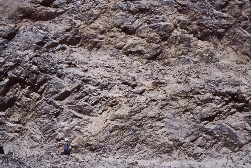
Figure 39. The alteration of rocks at Okorusu by early fenitization, early hydrothermal event, later by hydrothermal fluorite-depositing fluids, and finally by supergene oxidation fluids renders the already challenging geology even more challenging. The mine face in this view is typical of the difficulty in distinguishing areas of fenite (medium gray) from intrusive areas of carbonatite (light gray). A pit, Okorusu mine.
