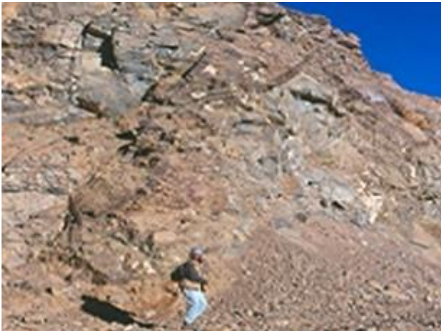
Figure 35. A nearly vertical dike of carbonatite (medium grey with white spots) with magnetite (black) rims, which is partly replaced by fluorspar ore (darker gray) that retains those magnetite rims. A pit, Okorusu.
