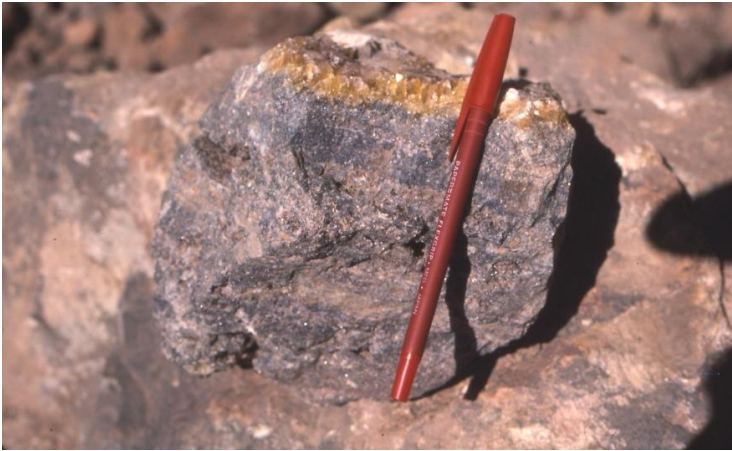
Figure 10. Hand specimen of vug-filling yellow fluorite (top crystal coating) deposited on massive purple replacement fluorite (main portion of hand specimen). 1710 level, B open pit, Okorusu Mine.
